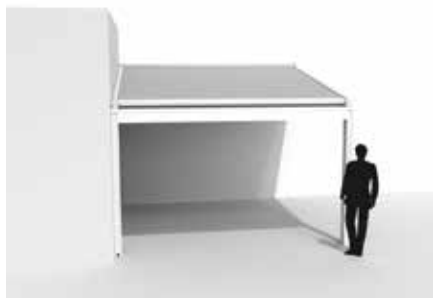
Construction situation 3 - Against rear and left structure
