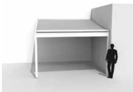
Construction situation 4 - Against rear and right structure
