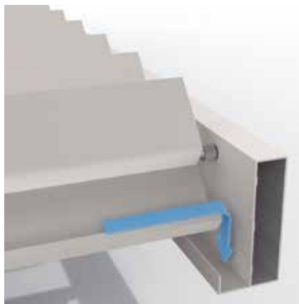
The Algarve Line can process a precipitation flow rate corresponding to a rain shower with an intensity of 144 mm/h to 180 mm/h that lasts max. 2 minutes. This type of rain shower occurs approx. every 10 years. (Cf. Belgian rain statistics: standard NBN B 52-011)
